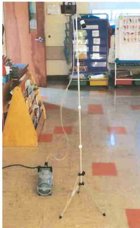
Typical PCM Air Sample Set-up
